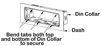
2. Connect to the radio's harness and antenna jack. Verify clearance; then gently insert the radio into the DIN Collar until both sides lock.
