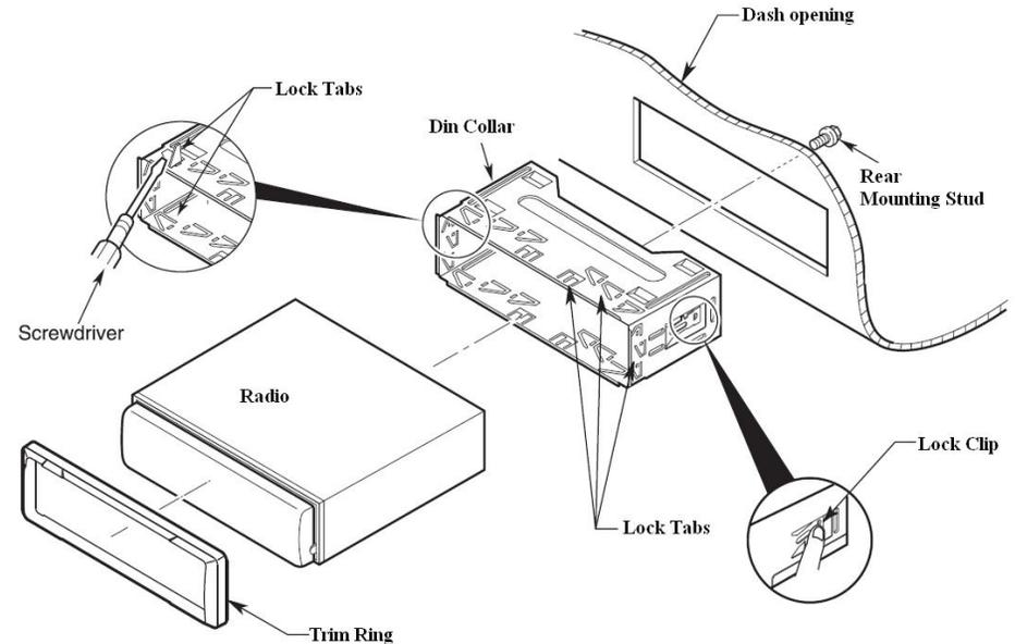
2. Route all cable through the DIN collar and make all the necessary rear connections with the radio. Verify clearance; then gently insert the radio into the DIN Collar until both sides are locked. Secure rear mounting stud for additional support.
